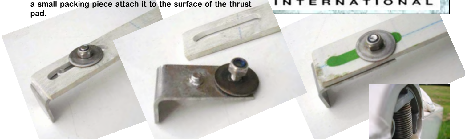
Pictures left to right Rear beam thrust pad and inside of hull contact Rear beam clip and leaf spring Adjustment slot filled to prevent creep Rear beam and clip in correct position
