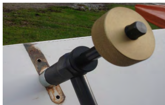
Below : Rivet nut and tool ready and in position to pull up (commercial rivet nut tool shown)
