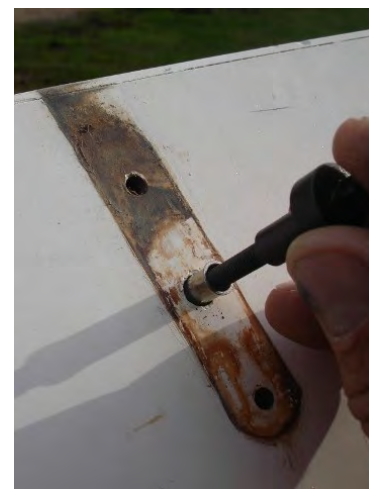
Right : Rivet insert being tested in hole for size
