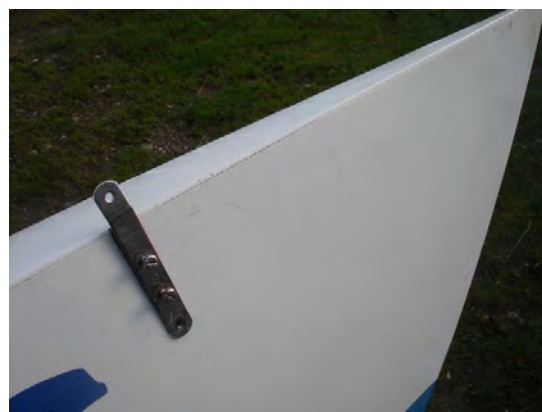
Above : Bow with bridle plate being re- moved
