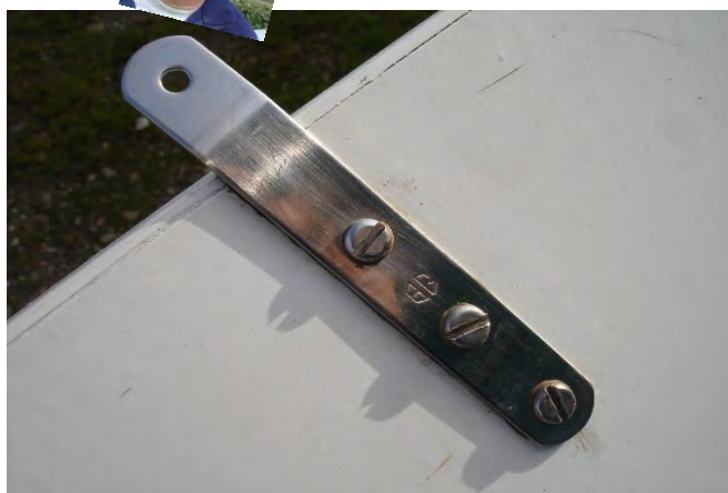
All three screw holes replaced with rivet nut and new bridle plate fitted
