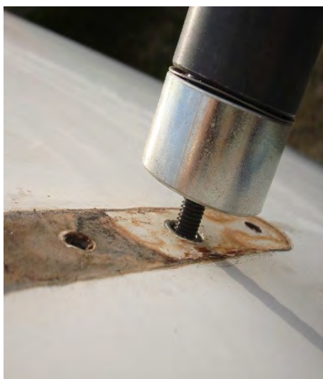
Below : Rivet nut in position with two more to do
