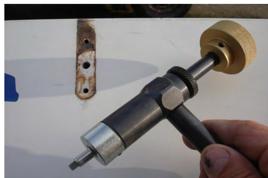
Above : Rivet fitted to rivet tool ready for use
